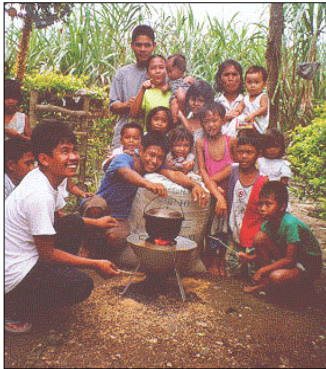
Photo 7. Communities in the Philippines are extremely interested in the LT-2000 stove. Fueled by residual hulls from rice production, this low-cost stove produces modest levels of smoke, is simple to start, and has a high heat output. Rice hull has the lowest annualized cost of the purchased fuel systems in the Philippines (Figure 7)
