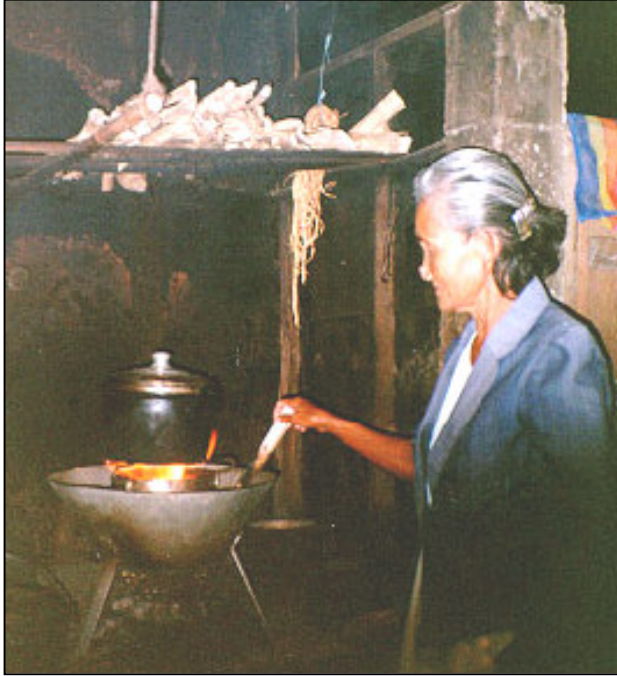
Photo 8. High efficiency stoves completely burn the fuel being used and effectively transfer the heat to the pot, thus reducing the amount of fuel needed for cooking. An important fuel saving feature is an adjustable heat output, for boiling then simmering rice. Sufficient energy is needed to replace heat losses during the latter part of the cooking cycle. Greater control of heat output would improve user acceptance of improved biomass cooking stoves.
