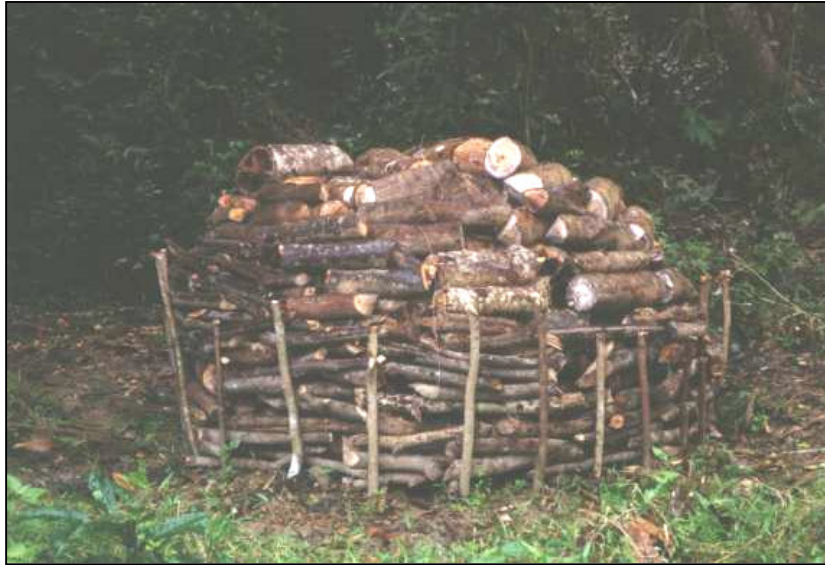
Photo 1. Native forests have been depleted by using wood for household cooking and by its conversion to charcoal (as shown in the above photo). Inefficient production systems and inefficient charcoal stoves mean that only about 5% of the wood energy is recovered as useful heat for cooking. There is a large, illegal charcoal trade that persists in the Philippines. Modernizing the charcoal industry and developing new cooking systems would reduce this trade.
