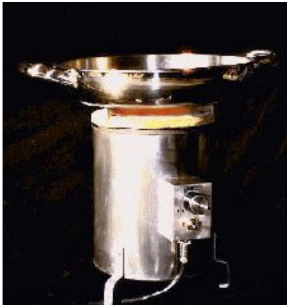
Photo 9: Prototype CPC Turbo (Wood-Gas) Stove suitable for burning pellets (Reed and Larson, 1996)
