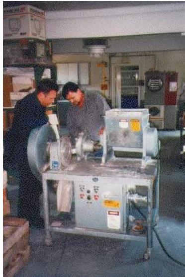
Figure 2. The 2HP California Pellet Mill-CL Type 5 lab model pelleter used in the studies
